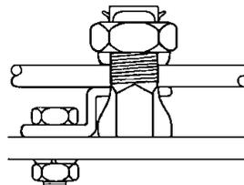
BL Series is tin-plated for use on aluminum pool structure. Use of oxide-inhibitor is recommended.
